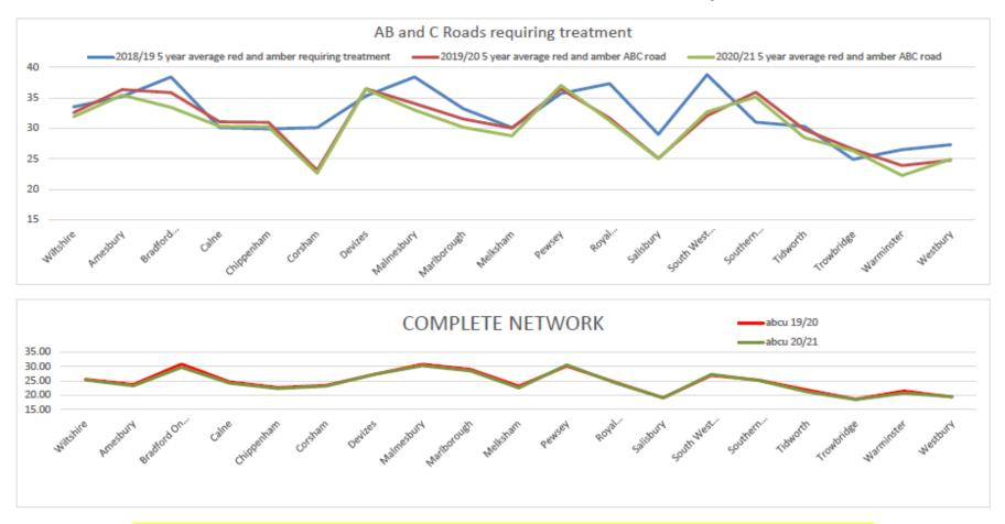
A 5 year average is used to monitor the condition of the network due to the surveying regime of undertaking a 50% network length
